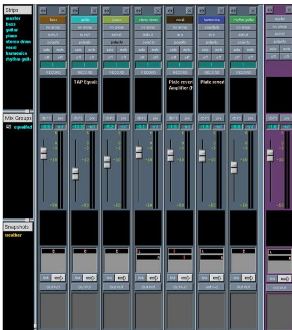
Figure 3. In the Mixer panel, think of audio data moving from the top down through each track strip.
